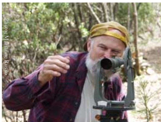
Jerry uses the transit to locate the western boundary of the Weller Natural Preserve.
